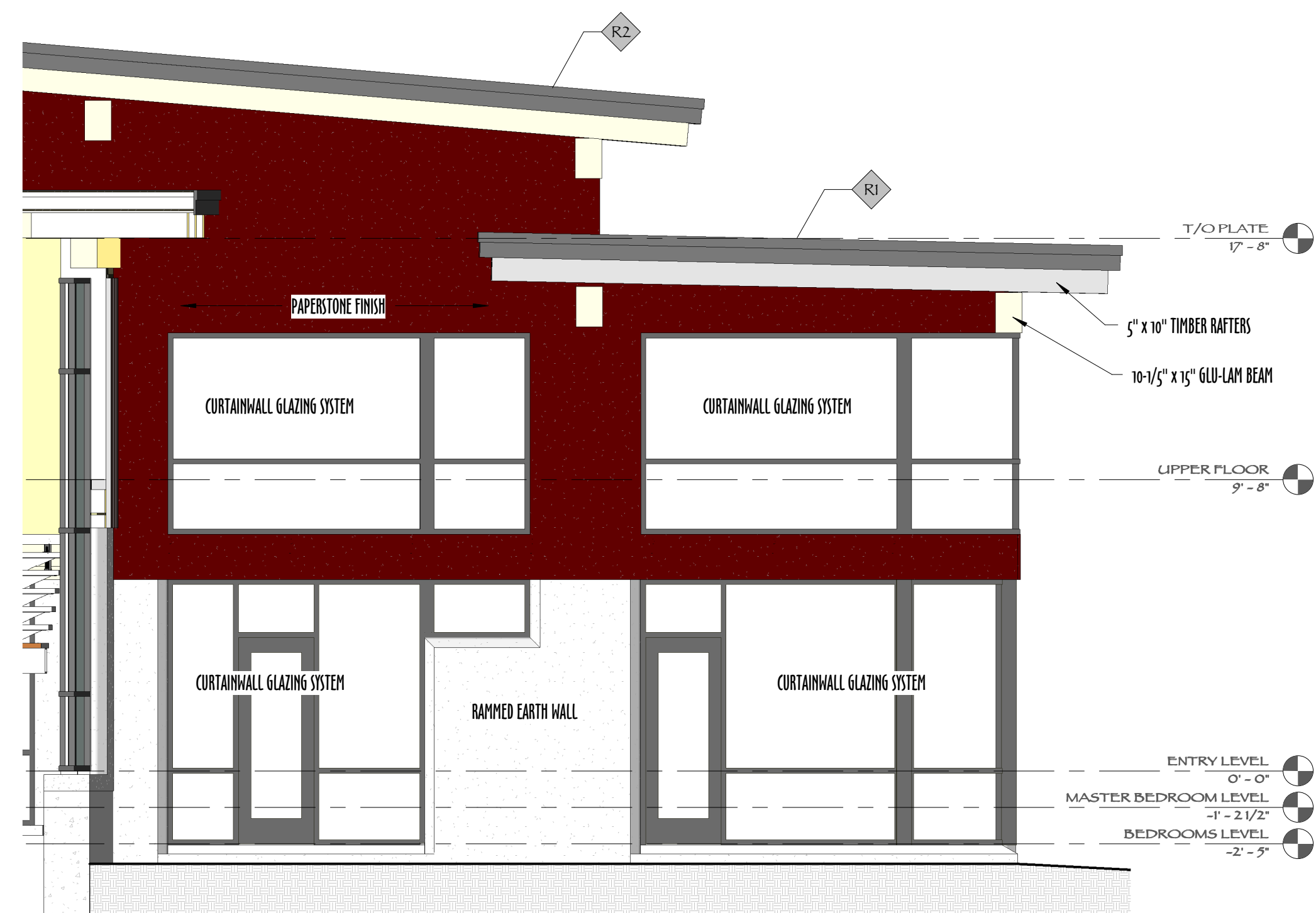
5 PARTIAL ELEVATION @ BEDROOM WING 1/4" = 1'-0"
